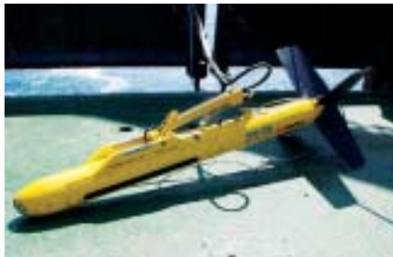
Typical sidescan sonar fish. The tow fish transmits and receives sound as it is towed behind the research vessel to produce a 'photograph-like' image of the seabed. DARD sidescan sonar system
