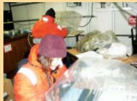
Sediment cores are sectioned in a nitrogen atmosphere to obtain porewater. This work is conducted in a cold room with temperatures equal to those on the seabed – making it necessary to wear winter clothing in the tropics!
