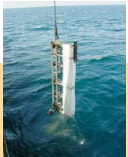
The benthic boundary layer sampler (BBLs) allows deep water to be collected short distances above the undisturbed seabed.
